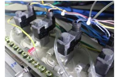
Vacuum transformation of the robot arm for sucking batteries: The original vacuum generator is removed, and the vacuum is directly provided by the factory vacuum pump. Only the solenoid valve is needed to control the on-off of the vacuum source, which can avoid the leakage loss of compressed air and improve production efficiency.
